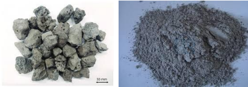
Figure 2. A steel making slag, EAF slag lumps (right), EAF slag powder (left).
