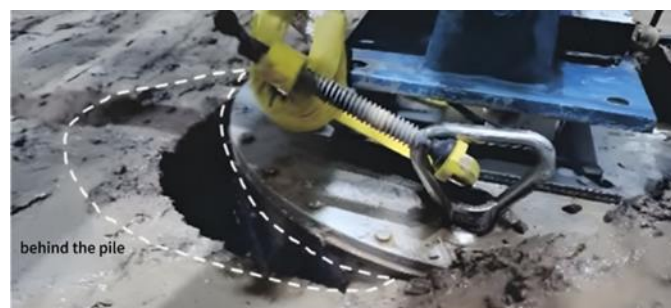
Figure 3. Separation phenomenon of soil behind the foundation[27]
