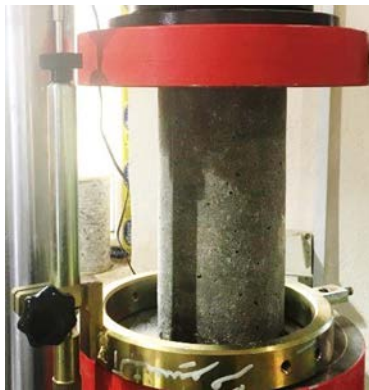
Fig. 5. Cylindrical test specimen under uniaxial pressure
