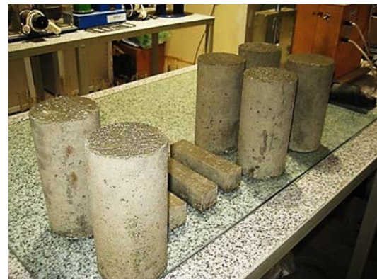
Fig. 3. Fabricated cylindrical and cuboid test specimens
