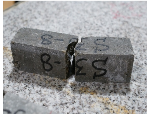
Fig. 8. Failure at midspan of a specimen under flexural test
