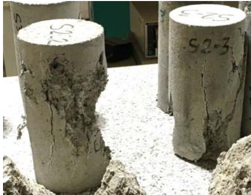
Fig. 7. Crushing patterns in specimens under compressive test
