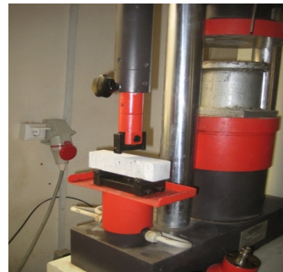
Fig. 6. Three-point flexural testing of a concrete specimen
