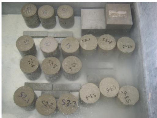
Fig. 2. Test specimens in the curing pond
