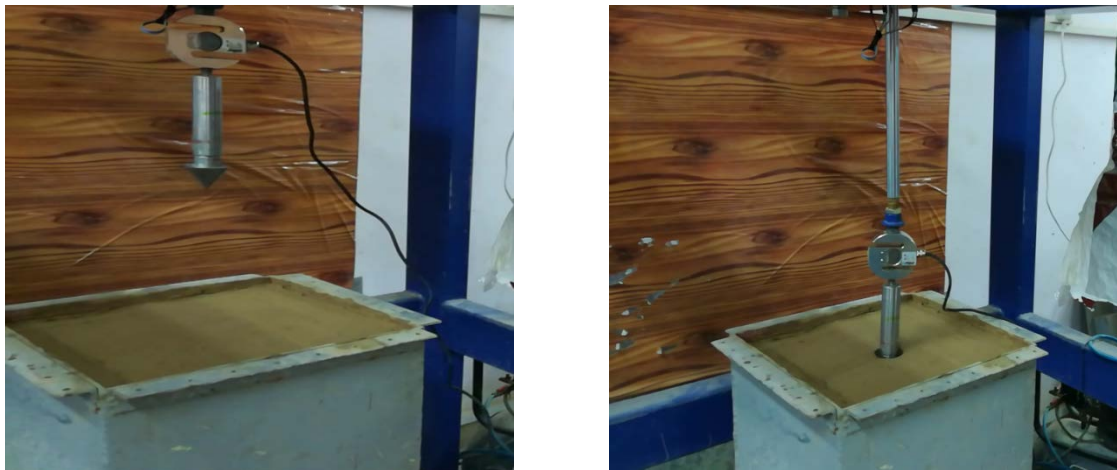
Fig. 6. Measuring device for soil shear resistance.
