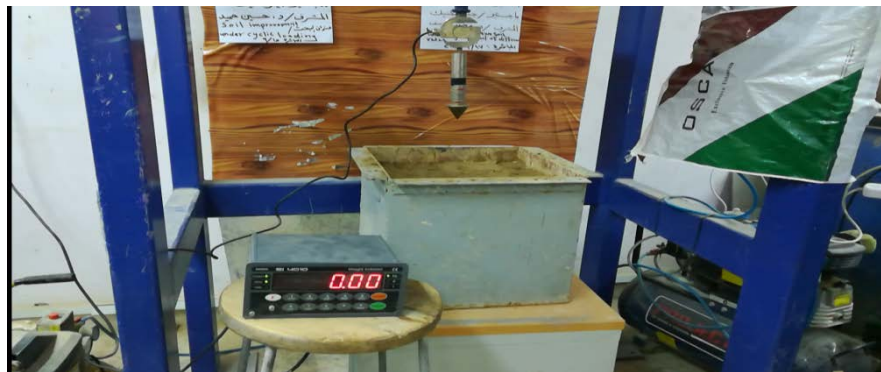
Fig. 10. Manufactured apparatus for measurement of soil strength.
